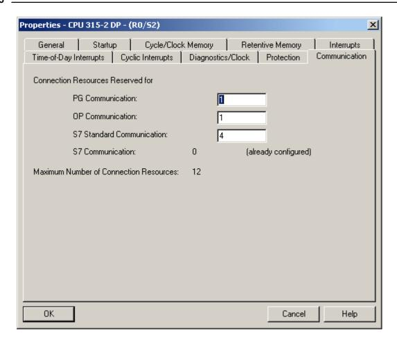
3. Configure the desired number of **PG/OP** and **PC (S7 Communication)** connections.
