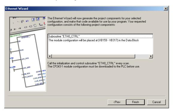
2. To review what the Ethernet wizard produced, double-click **ETHO\_CTRL** under the **Program Block**. All **TSAPs** configured are listed for future reference. Remember, the **Local TSAP** below is the **Remote TSAP** in the OPC server and the remote TSAP below is the Local TSAP in the OPC server.
