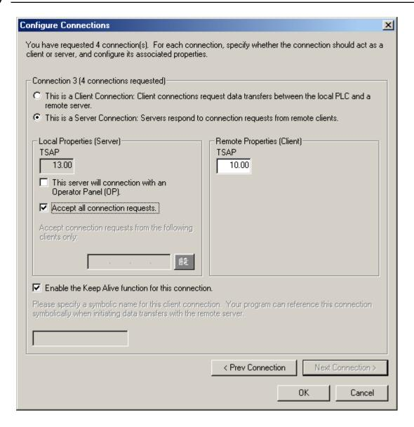
That completes the configuration of the four connections that were selected.  $\label{eq:configuration}$
