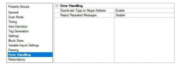
**Deactivate Tags on Illegal Address**: When enabled, the driver stops polling for a block of data if the device returns Modbus exception code 2 (illegal address) or 3 (illegal data, such as number of points) in response to a read of that block. When disabled, the driver continues to poll that data block. The default setting is enabled.
