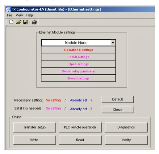
4. Next, fill in the minimum required configuration information for the FX3U-ENET block. Select a module from the first drop-down list, and then click **Operational Settings**. The settings should be similar to those shown in the image below.
