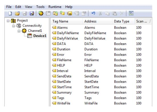
Note: Generated tag names are essentially the same as the tag names in InTouch. Minor name modifications may be required and are indicated in the Event Log when they occur. The addresses in the OPC server are the same as the tag names in InTouch.
