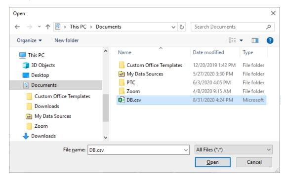
In this example, the file in an InTouch project folder called "DB.CSV" has been selected. Once **OK** is clicked, the full path and file name is automatically placed in the InTouch CSV file box.
