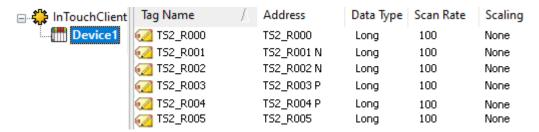
In this example, tags TS2\_R001 and TS2\_R002 are placed in Notified Mode regardless of the device-level settings. Tags TS2\_R003 and TS2\_R004 are placed in Polled Mode regardless of the device-level settings. All other tags shown above use the default mode specified in Device Properties.
