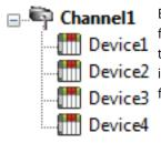
Each device appears under a single Honeywell UDC Ethernet channel. In this configuration, the driver must move from one device to the next as quickly as possible to gather information at an effective rate. As more devices are added or more information is requested from a single device, the overall update rate begins to suffer.
