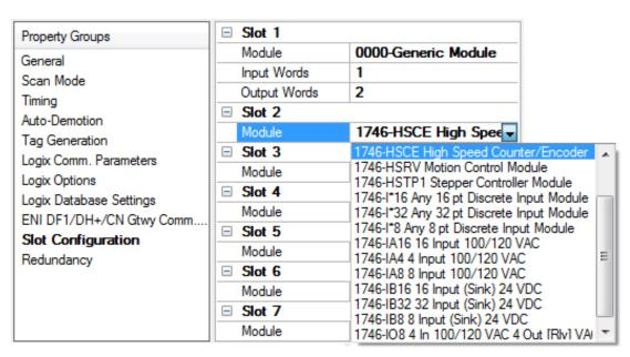
**Slot** *n*: the physical slot being configured. Use the plus icon to expand the properties.
