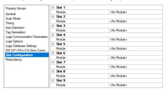
**Slot** *n*: the physical slot being configured. Use the plus icon to expand the properties.
