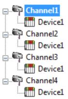
Each device can be defined under its own channel. In this configuration, a single path of execution is dedicated to the task of gathering data from each device.
