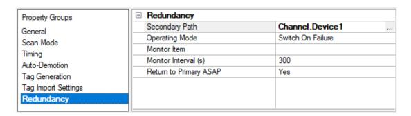
**Secondary Path**: Specify the explicit, unaliased path to the device serving as backup should the primary device fail. The valid format is *<channel>.<device>*. The default setting is blank.
