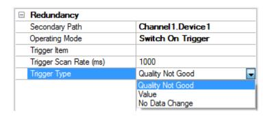
**Trigger Item:** Specify a fully qualified dynamic or static item reference. This item is used as the source of the trigger and is regularly evaluated at the configured scan rate to determine if a switchover is required. To choose a static item reference defined in the server,
