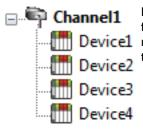
Channel1 Each device appears under a single channel. In this configuration, the driver must move from one device to the next as quickly as possible to gather information at an effective rate. As more devices are added or more information is requested from a single device, the overall update rate begins to suffer.
