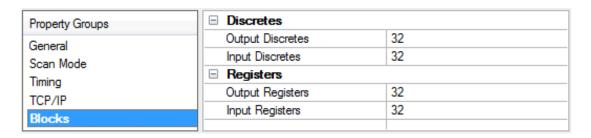
**Output**: The output block size for ELC memory types S, Y, To, M and Co may be between 8 and 1024 in multiples of 8. The default is 1024.
