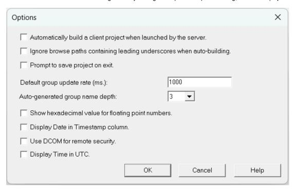
**Automatically Build a Client Project When Launched by the Server**: When checked, the OPC Quick Client will automatically build a client project with all the tags in the OPC server when it is launched from the OPC server. The default setting is checked.
