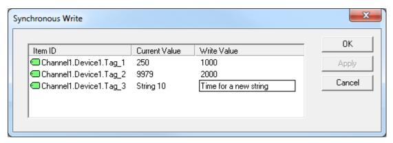
Note: Both types of writes utilize the same dialog. The dialog displays the current value at a 100 millisecond refresh rate. To send the data to the server, enter the data to write in the Write Value column and then press Apply. To apply the write and close the dialog, click **OK**. To cancel the operation, click **Cancel**.
