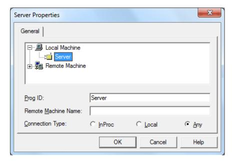
**Prog ID**: This parameter specifies the Prog ID of the OPC Server to which the client will connect. Use the tree display to browse for registered servers. The Prog ID field can be automatically updated by double-clicking on any registered server.
