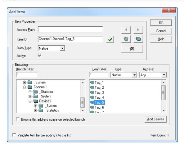
**Access Path**: This parameter is required by some OPC servers to complete an item definition. To determine whether an access path is needed, refer to the OPC server's help documentation.
