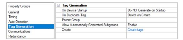
On Property Change: If the device supports automatic tag generation when certain properties change, the On Property Change option is shown. It is set to Yes by default, but it can be set to No to control over when tag generation is performed. In this case, the Create tags action must be manually invoked to perform tag generation.
