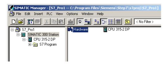
2. If this is a new Simatic project, add the necessary modules to the **Rack** in HW Config. For the Siemens TCP/IP Ethernet Driver to communicate with the CPU, there will need to be at least one Ethernet module capable of **S7 Communications**. This may be built into the CPU.
