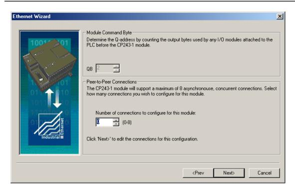
Note: The number of connections selected determines how many simultaneous connections the PLC can support. When intending to have only one OPC server talking to the PLC, set up only one connection. This will ensure the best performance for the OPC server. When intending to have more than one active connection to the PLC, use multiple connections. Keep in mind, however, that the performance of the module will be impacted as each connection is used.
