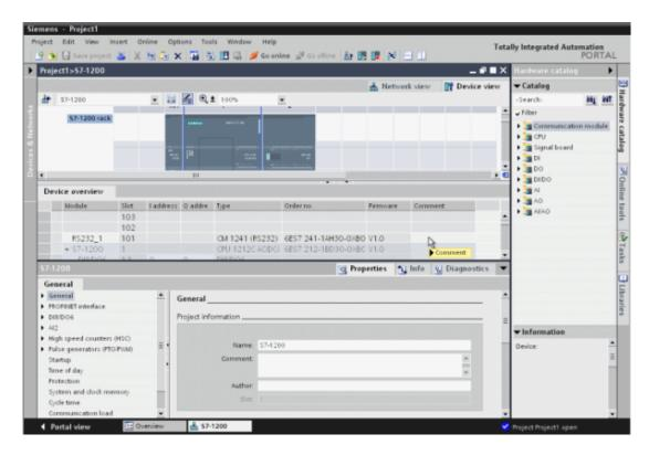
11. Once finished, view the project tree. Locate **Program Blocks** and **PLC Tags** and then configure the addresses that will be used in the PLC project.
