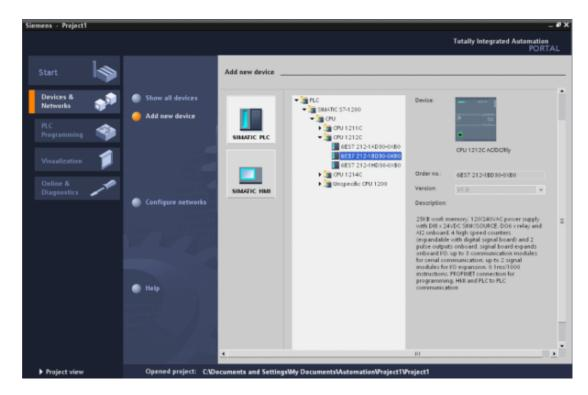
10. Next, select the device's configuration and then click **Add device**. This will invoke the Project View, where the device's hardware can be further configured.
