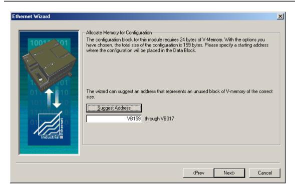
• **Note:** It is recommended that the Micro/WIN software pick this location for the application. If a CRC was not generated for the configuration data, please take steps to ensure that no other aspect of the PLC program will overwrite this area of memory.
