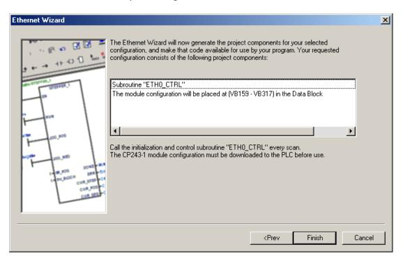
2. To review what the Ethernet wizard produced, double-click **ETH0\_CTRL** under the **Program Block**. All **TSAPs** configured are listed for future reference. Remember, the **Local TSAP** below is the **Remote TSAP** in the OPC server and the remote TSAP below is the Local TSAP in the OPC server.
