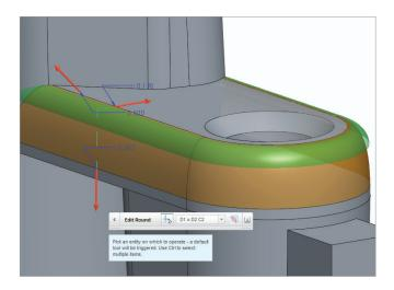
Quickly move geometry using the intuitive 3D dragger with automatic round and chamfer handling.
