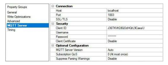
Host: The IP address or host name of the MQTT server to connect. The default is localhost.
