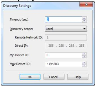
**Timeout**: This parameter specifies the length of time that the driver waits for all "I-Am" responses to the initial "Who-Is" discovery request. It is also used to timeout non-responsive devices when requesting device names. The default setting is 3 seconds.
