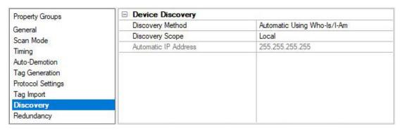
**Discovery Method**: Select how the driver obtains the required device properties.
