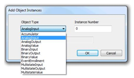
**Object Type**: Select the BACnet object type of the object identifier that is configured with intrinsic or algorithmic event reporting or is configured as the object property referenced in an event enrollment object. The default selection is AnalogInput.
