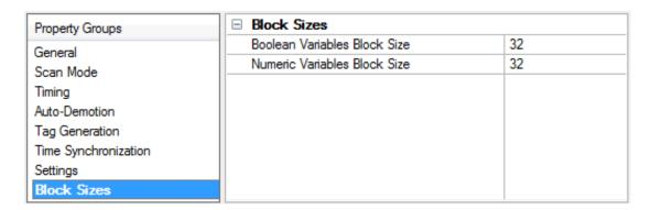
**Boolean Variables Block Size**: Specify the output and input coils. Coils can be read from 8 to 2000 points (bits) at a time. A higher block size means more points will be read from the device in a single request. The block size can be reduced to read data from non-contiguous locations within the device. The default setting is 32.
