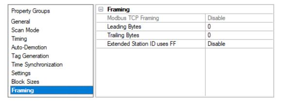
**Modbus TCP Framing**: When enabled, this option communicates with native Modbus TCP devices using Ethernet Encapsulation. For more information, refer to "Using Ethernet Encapsulation" below.
