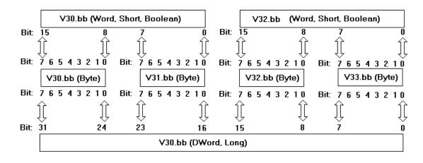
• Note: V30.10@bool, V30.2@byte, and V30.26@DWord all reference the same bit in the controller.
