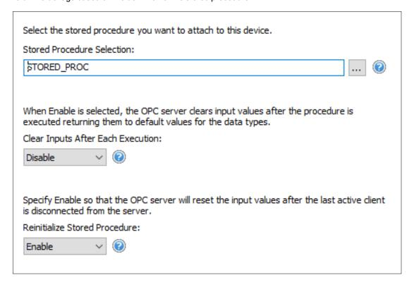
**Stored Procedure Selection**: This property specifies the stored procedure that will execute when a user writes to the Execute internal control tag.
