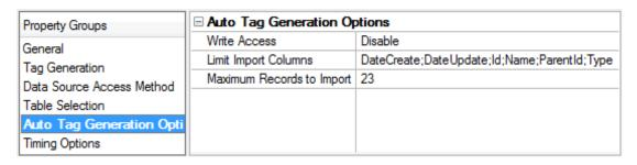
Write Access: This property specifies the default Write privileges when automatically generating tags. It only sets the tag's access privileges to Read/Write in the server: it does not affect the field's access privileges in the database.
