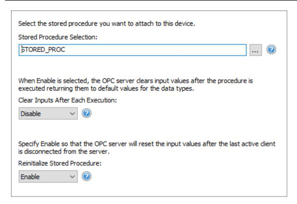
Clear inputs after each execution: When enabled, the OPC server clears the input values after the stored procedure is executed, returning them to the default values for the data types. The default setting is disabled.
