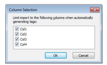
• Maximum Records to Import: This property specifies the maximum number of records to import. The default setting will automatically generate tags for all records in the table, but users can limit the number is desired. This property only applies to Fixed Table. The default setting is 0.
