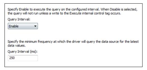
**Query Interval**: When enabled, this property enables the query to run each time the query interval elapses. When disabled, the query will not run unless a write to the Execute internal control tag occurs. The default setting is enabled.
