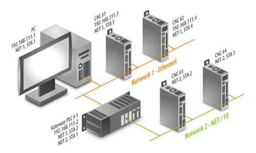
The gateway has an AJ71QE71 Ethernet module and NET/10 module. CNC 1 and CNC 2 have an AJ71QE71 Ethernet module and NET/10 module. CNC 3 and CNC 2 have a NET/10 module. In this example, four devices are created in the server project using the Device IDs listed in the table below.
