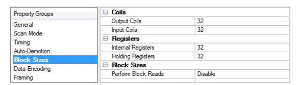
**Coils (8-2000 in multiples of 8):** These properties specify the output and input coils. Coils can be read from 8 to 2000 points (bits) at a time. A higher block size means more points will be read from the device in a single request. The block size can be reduced to read data from non-contiguous locations within the device. The default setting is 32.
