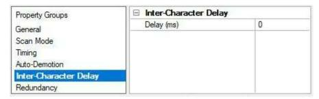
**Delay**: Specify the controlled delay between each character the driver sends to an Omron device. The valid range is 0 to 200 milliseconds. The default setting is 0 milliseconds.
