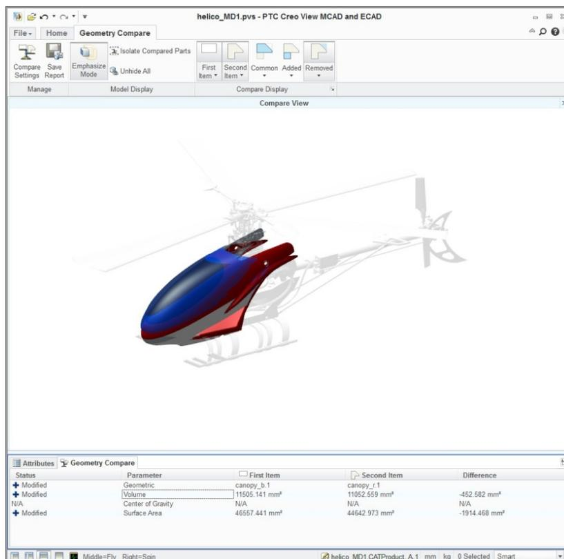
**Figure 1—Comparing 3D Model Variants with PTC Creo View MCAD**
