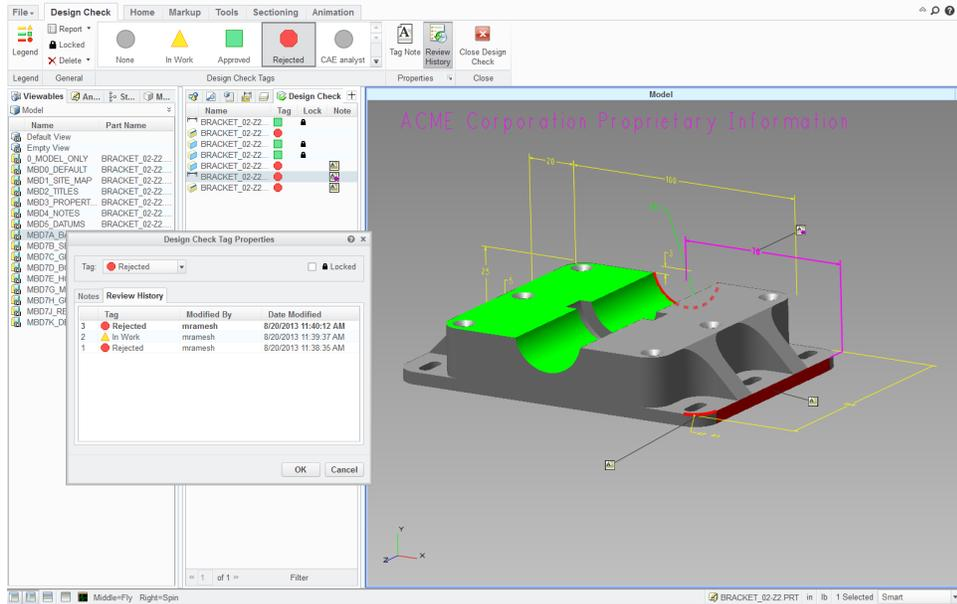
**Figure 2—Exploring the Results of PTC Creo View Design Check**
