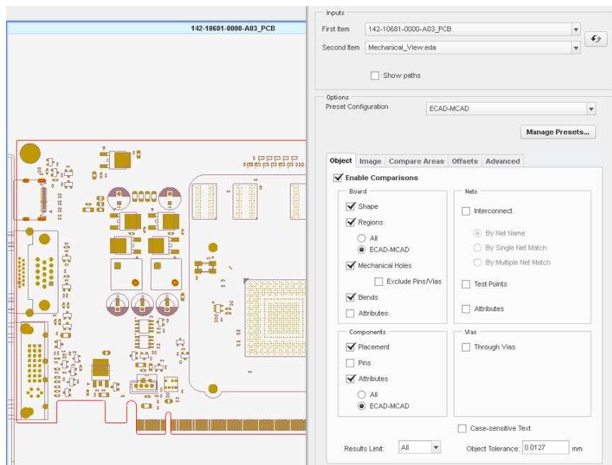
Figure 6—Performing an ECAD-MCAD Compare
