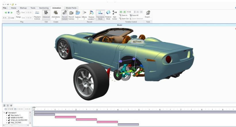
**Figure 4—Animating a Disassembly using PTC Creo View Animator**
