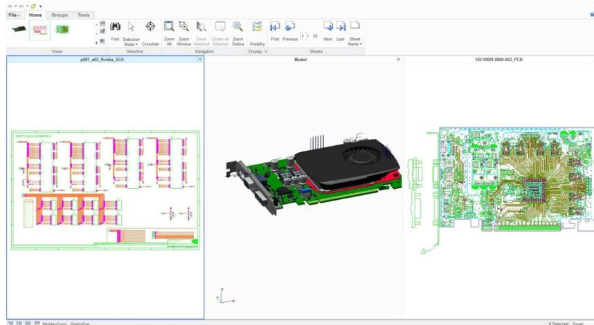
**Figure 5—Displaying an Electronic Schematic, 3D PCB, and PCB Layout Views**
