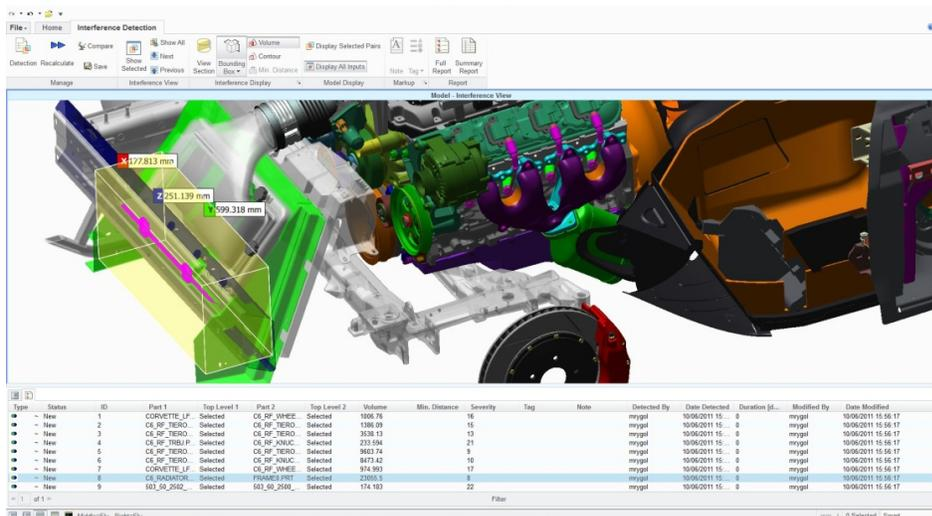
**Figure 3—Investigating an Interference using PTC Creo View Interference Analysis**
