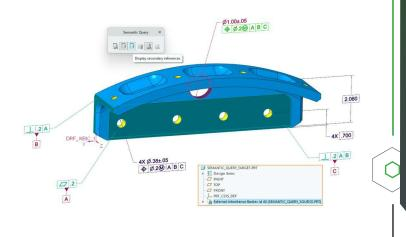
For years, engineers used 2D drawings to deliver product manufacturing information-even as they designed models in 3D. Now, using **Model-Based Definition (MBD)**, engineers embed product data directly into the 3D model, creating a single, reliable source of truth which, as a result, prevents errors and saves on time.
