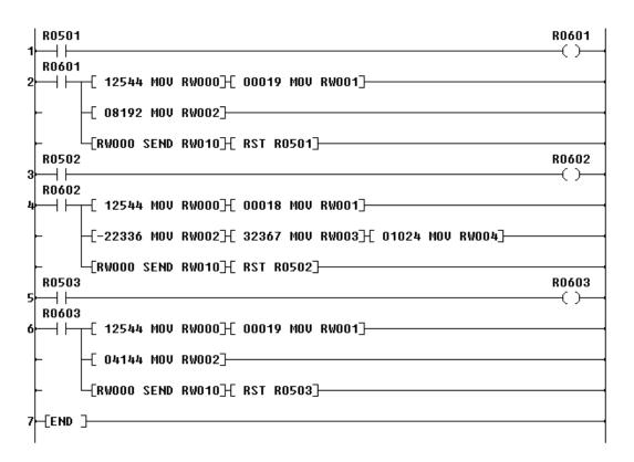
The first block of code at rung 2 places the PLC in Standby Mode when bit R0501 is set. This must be done before the IP and port can be set. The second block of code at rung 4 sets the IP and port number when bit R0502 is set. The final block of code at rung 6 puts the PLC back in Run Mode when bit R0603 is set.
