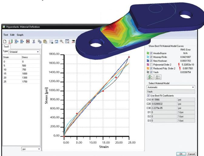
PTC Creo Advanced Simulation Extension simulates nonlinear, hyper-elastic behavior and allows you to define material properties using your own test data.
