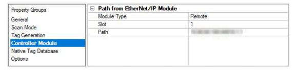
**Module Type**: Verify if the device is Local (part of the simulated EtherNet/IP Module) or Remote (which require a slot number for EtherNet/IP routing). There can be one Local CPU and up to fifteen Remote CPUs.
