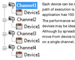
Each device can be defined under its own channel. In this configuration, a single path of execution is dedicated to the task of gathering data from each device. If the application has 100 or fewer devices, it can be optimized in this manner.
