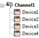
Channel1Each device appears under a single channel. In this configuration, the driver must<br/>move from one device to the next as quickly as possible to gather information at an<br/>effective rate. As more devices are added or more information is requested from a<br/>single device, the overall update rate begins to suffer.
