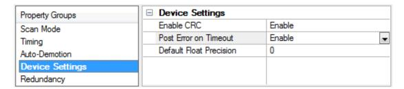
**Enable CRC**: When CRC is enabled, the Contrex Serial Driver appends a 16-bit CRC value at the end of each data transmission. The driver calculates and compares the 16-bit CRC value received from the controller for any errors. Users should determine if CRC is enabled on the controller and set this parameter accordingly. The default is Enable.
