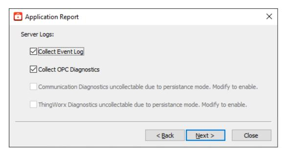
The Event Log collection interface is divided into two sections, allowing collection of server logs and LinkMaster logs. If either product is not installed, the section is disabled.
