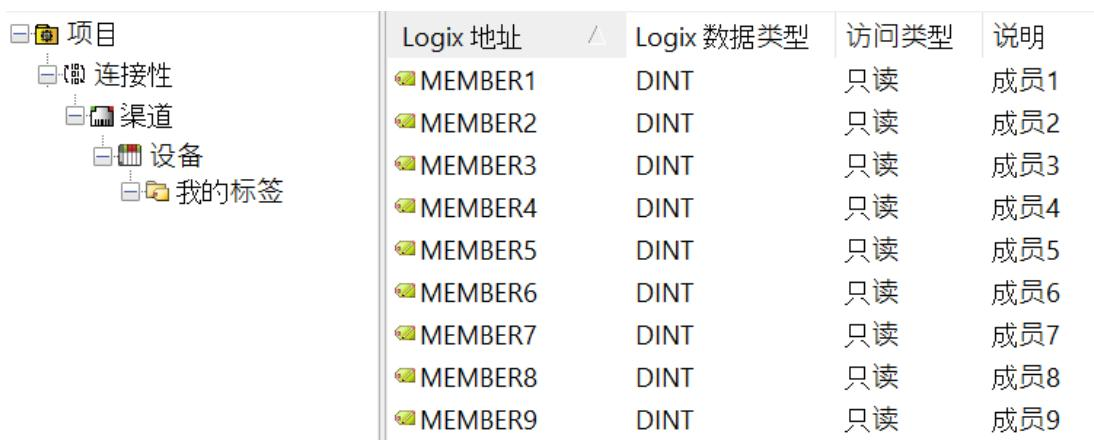
The screenshot shows the project tree on the left with nodes for Project, Connection, Channel, Device, and My Tags. On the right is a table mapping Logix addresses to data types and access levels:
