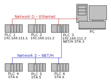
If PLC 1, PLC 2 and PLC 3 have QJ71E71-100 Ethernet modules configured with IPs 192.168.111.1, 192.168.111.2 and 192.168.111.3 respectively. In addition to the Ethernet module, PLC 3 also has a QJ71BR11 NET/H module configured as station 3. Assume that PLC 4, PLC 5 and PLC 6 have NET/H modules configured as stations 4, 5 and 6 respectively.
