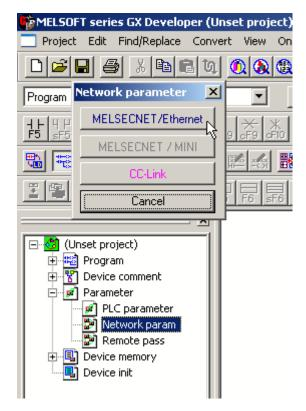
4. Fill in the required information for the Ethernet module. Although the network type must be Ethernet, other settings will depend on the particular application. The example below is for station 1 on network 1. The
