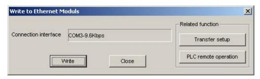
Note: There must be a serial connection to the FX3U PLC. The configuration settings are written to the PLC via this serial link. Also make sure that the communication parameters are correct. Settings can be checked by clicking Transfer Setup or be selecting Online | Transfer Setup from the main menu.
