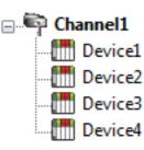
Each device appears under a single channel. In this configuration, the driver must move from one device to the next as quickly as possible to gather information at an effective rate. As more devices are added or more information is requested from a single device, the overall update rate begins to suffer.
