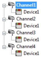
Each device can be defined under its own channel. In this configuration, a single path of execution is dedicated to the task of gathering data from each device. If the application has 64 or fewer devices, it can be optimized as it is shown here.
