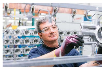
Networked production technologies guide workers through the individual production steps, which increases productivity and lowers the reject rate. (Image source: Knorr-Bremse AG)
