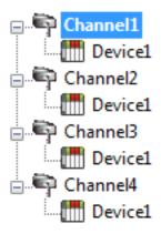
Each device can be defined under its own channel. In this configuration, a single path of execution is dedicated to the task of gathering data from each device. If the application has 256 or fewer devices, it can be optimized exactly how it is shown here.
