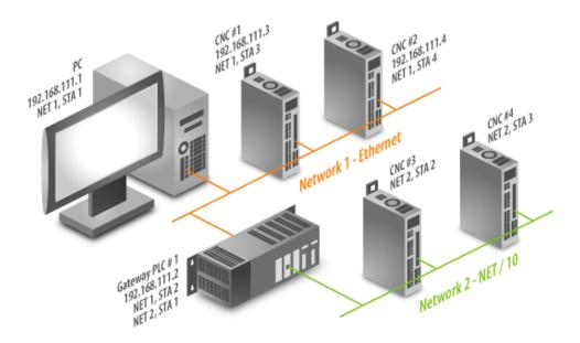
The gateway has an AJ/1QE71 Ethernet module and NET/10 module. CNC 1 and CNC 2 have an AJ/1QE71 Ethernet module and NET/10 module. CNC 3 and CNC 2 have a NET/10 module. In this example, four devices are created in the server project using the Device IDs listed in the table below.
