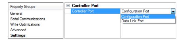
**Controller Port**: Specify the port to which the Micro-DCl unit to connect. The **Configuration Port** should be selected when connecting to the front DIMM port on the device. The **Data Link Port** should be selected when using an RS485 connection through the RS485 interface on the back of the device.
