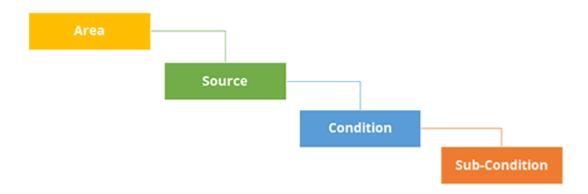
**Area**: Areas are the root of the hierarchy and are used strictly for organizational purposes. They can be sections of a plant, sub-sections, parts of a machine and so forth. Areas may contain other areas in addition to sources.
