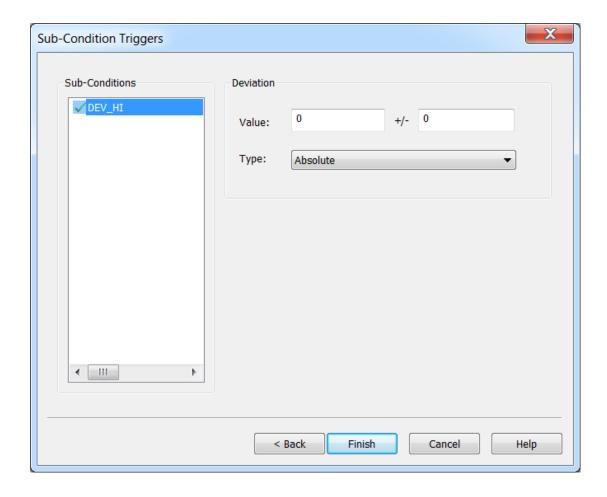
**Value**: The fixed point on which the deviation is based. Any real number is supported.
