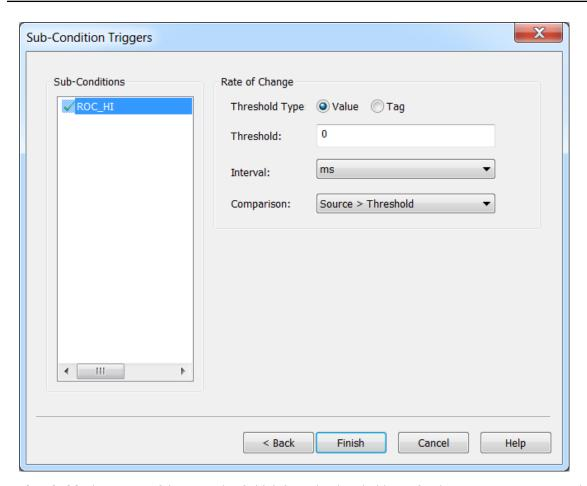
**Threshold**: The source of the ROC. This field defines the threshold ROC for the comparisons. It is a value or an OPC server tag address. If the threshold is a value, it represents a rate of change in units/time. If the threshold is a tag, it is the ROC of the OPC server tag. All OPC server tags are available except complex and array tags.
