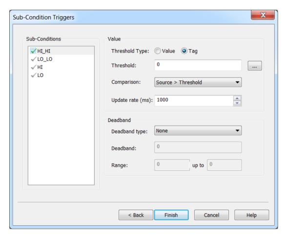
**Threshold**: A static value or tag which is compated to the data updates from the parent source. If the threshold is a tag, any OPC server tag is available aside from array tags and complex tags.
