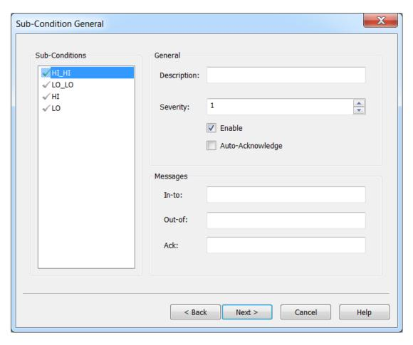
**Description**: The description of what the sub-condition is for. This description is sent to OPC AE clients when they query for the state of a condition. The maximum length is 1024.
