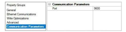
**Port**: Specify the port number to be used by the devices on the local Ethernet network. FINS requires that the source and destination port number be the same. The valid range is 1 to 65535. The default setting is 9600.
