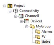
**Auto Create** manually initiates the creation of automatically-generated OPC tags, and also forces the communications driver to reevaluate the device for possible tag changes. It can be accessed from the System Tags, thus allowing the OPC client application to initiate tag database creation.
