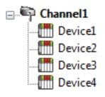
Each device appears under a single Yokogawa DXP Driver channel. In this configuration, the driver must move from one device to the next as quickly as possible to gather information at an effective rate. As more devices are added or more information is requested from a single device, the overall update rate begins to suffer.
