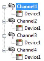
Each device can be defined under its own channel. In this configuration, a single path of execution is dedicated to the task of gathering data from each device. If the application has fewer devices, it can be optimized in this manner.
