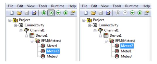
When creating meters, note that the DB1 protocol supports only a single meter and the DB2 protocol supports a maximum of 128 meters. This does not necessarily reflect the number of meters that can be created in the Total-flow device.
