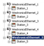
Each device can be defined under its own channel. In this configuration, a single path of execution is dedicated to the task of gathering data from each device. If the application has fewer channels, it can be optimized exactly how it is shown here.
