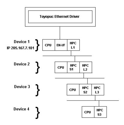
A routing command can only be issued through a maximum of four devices. Routing allows the Ethernet driver to request data from non-Ethernet devices. To request data from Device 3, the driver can route a command through Device 1 onto Device 2 then to Device 3.
