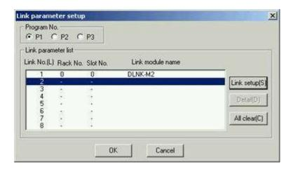
7. In the **Program No.** field, select the program that the configuration will be placed in. Click **Link Setup**.
