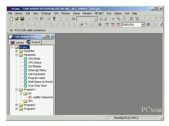
2. Read the existing program and parameters from the PLC by clicking on **CPU** | **Read Data**. Select the proper option.
