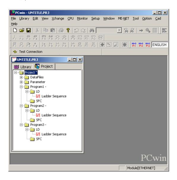
2. To setup the communication between PCWin and PC10G-CPU, click **Setup | Setup Communication Module**. If it is the first time configuring PCWin, select **Addition** and then make the selections as shown below.
