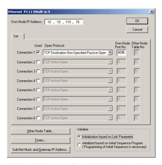
9. Click **Sub-Net Mask and Gateway IP Address** and specify the desired subnet and gateway settings.
