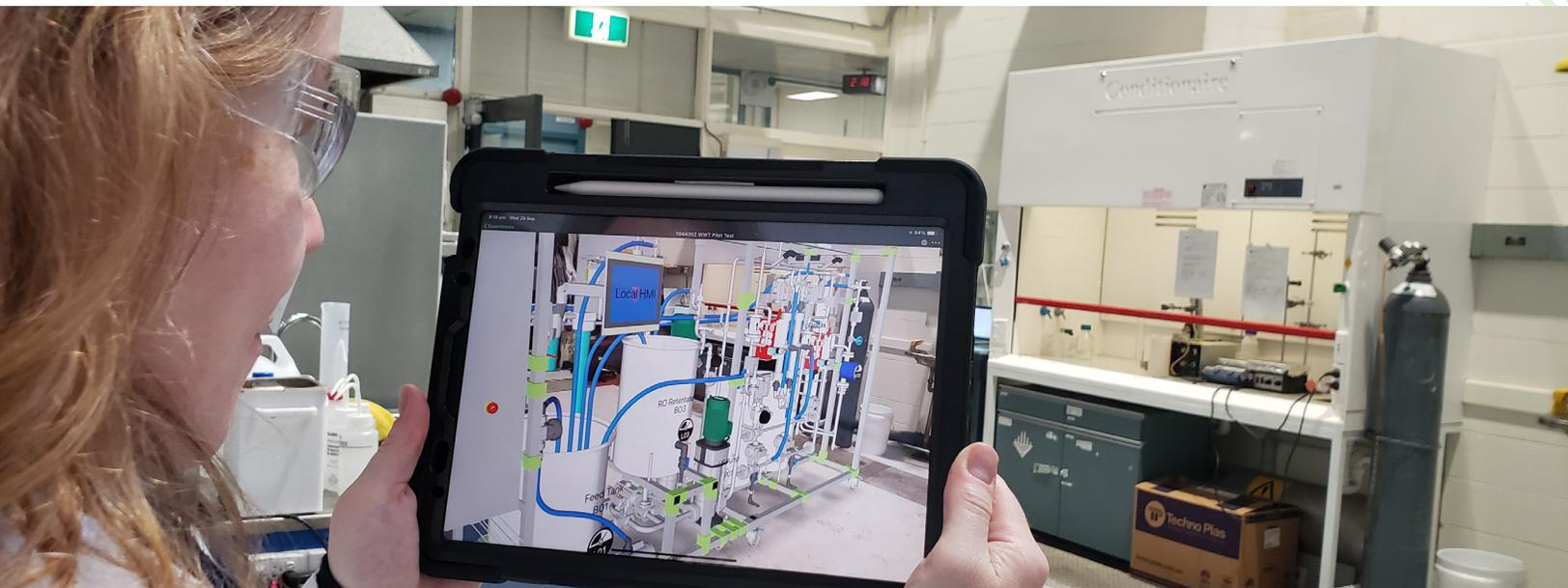
Those experiences will be connected to the Thingworx IoT/digital twin platform and Ansys simulations to create an AR-based Human Machine Interface (HMI) to expand on-site accessibility to the physical equipment via remote and simultaneous access to the digital twin.
