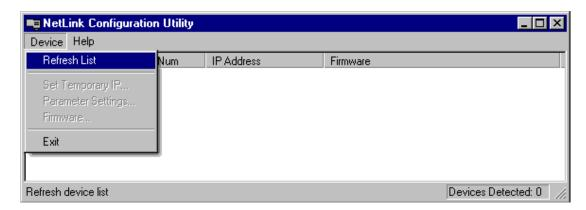
The main window displays a list of all NetLink devices detected. The view contains four columns:
