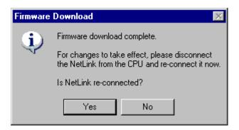
It is necessary to reconnect the device for the new firmware to be used. Click **Yes** when the NetLink is reconnected. The NetLink Configuration Utility pauses to allow the NetLink to complete its power-up sequence.
