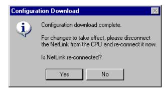
It is necessary to reconnect the device for this new configuration to be used. Click **Yes** when the NetLink is reconnected. The NetLink Configuration Utility pauses to allow the NetLink to complete its power-up sequence.
