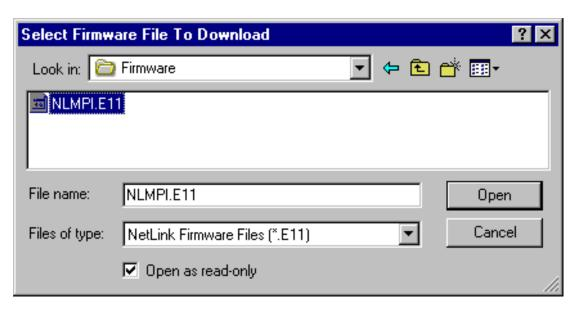
NetLink firmware files have a file extension of "E11." Once a file is selected, click the **Open** button to accept the selection.
