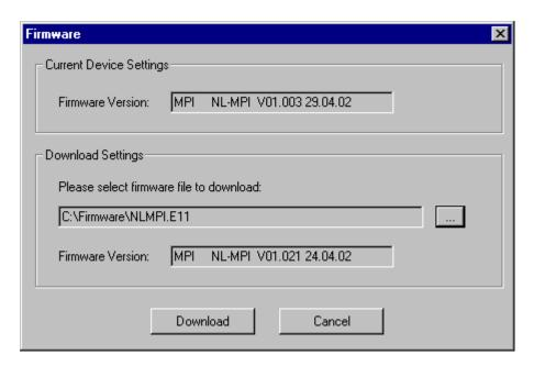
With a firmware file selected, a comparison can be drawn between the current firmware version and the selected firmware version.
