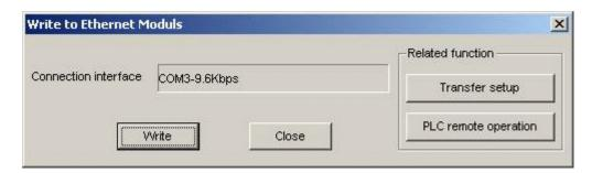
• Note: There must be a serial connection to the FX3U PLC. The configuration settings are written to the PLC via this serial link. Also make sure that the communication parameters are correct. Settings can be checked by clicking **Transfer Setup** or be selecting **Online** | **Transfer Setup** from the main menu.
