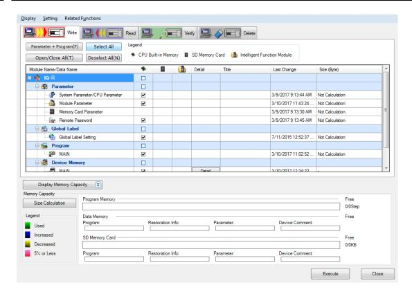
Note: Users must cycle the power on the PLC for the network parameter changes to take effect.
