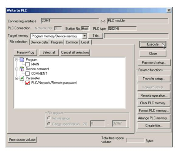
Note: Users must cycle the power on the PLC for the network parameter changes to take effect.
