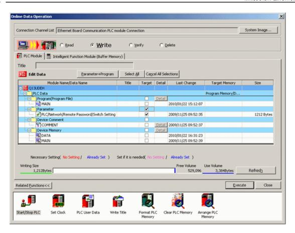
Note: Users must cycle the power on the PLC for the network parameter changes to take effect.
