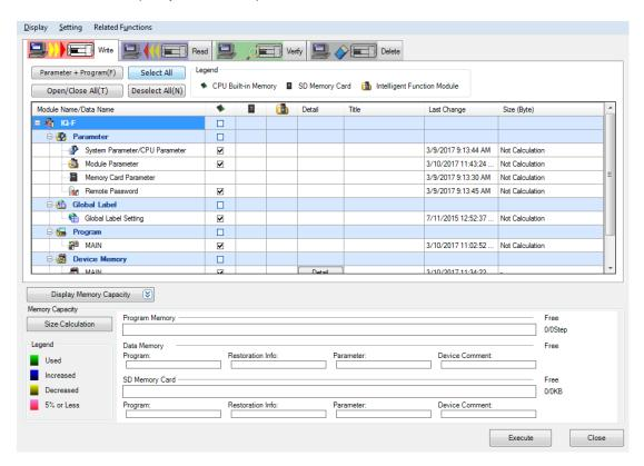
• Note: Users must cycle the power on the PLC for the network parameter changes to take effect.
