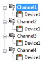
Each device can be defined under its own channel. In this configuration, a single path of execution is dedicated to the task of gathering data from each device. If the application has fewer devices, it can be optimized in this manner.
