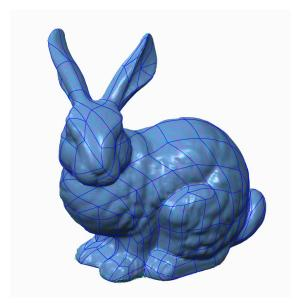
With Creo Reverse Engineering, you are able to capture valuable data without having the original CAD files. The above image shows the resulting facet model from a scanned point cloud of a rabbit. Verification tools ensure that the resulting CAD model accurately represents the scanned data. Finally, we have our complete model.
