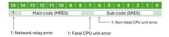
If bit 6 or 7 is ON, an error has occurred in the destination CPU Unit. If this occurs, refer to the operation manuals for the CPU Unit where the error occurred and then remove the cause of the error.
