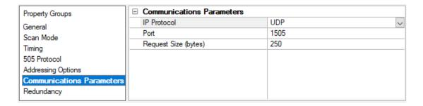
IP Protocol: This property specifies whether the driver should connect to the remote device using the User Datagram Protocol (UDP) or Transfer Control Protocol (TCP). This driver requires Winsock V1.1 or higher.
